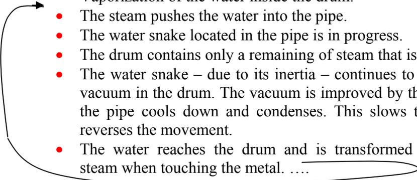
And this, until the flames extinguishes. Then the drum cools down, the steam condenses and we come back to the initial situation with drum and pipe full of water.
