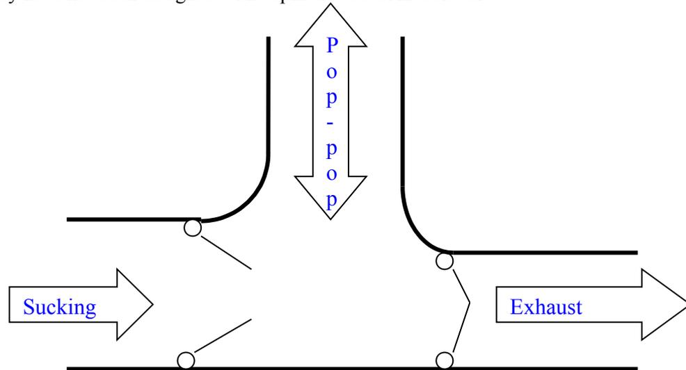
Note: For those who would be interested to do such an experiment, for the manufacturing a piece of thin plastic hose with a soft ironing on one end can do a cheap check valve with a very small inertia.
