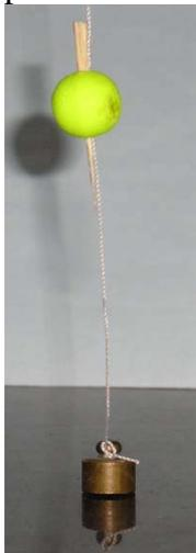
This mooring buoy consists in a weight (2g) laid on the tank bottom and a small polyurethane foam float held at an adjustable distance from the bottom thanks to a sewing thread and a little pin.
