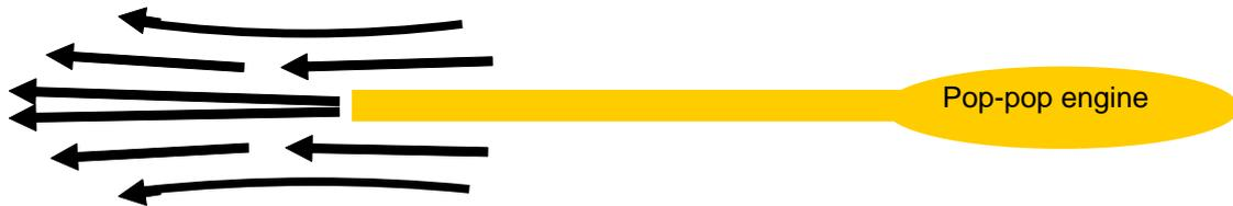
During the relaxation phase a low pressure is created at the nozzle end. To fill this "black hole" water comes from any direction.
