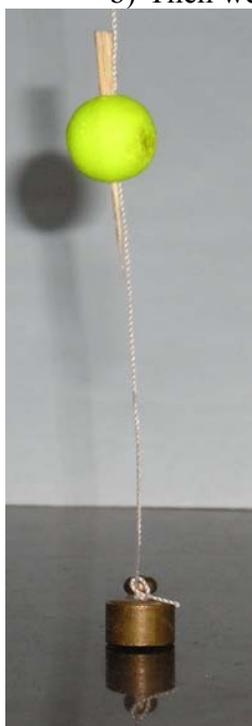
This device is made of a small weight (2g), a piece of sewing thread and a small polyurethane foam float (diameter 8mm) adjustable along the thread thanks to a little wedge. We placed this device in the tank at various places and we observed the inclination of the thread, and most of all the movements of the float. It was clearly visible that some water was re-circulated towards the target; therefore, the momentum was bigger than what it would have been in air.
