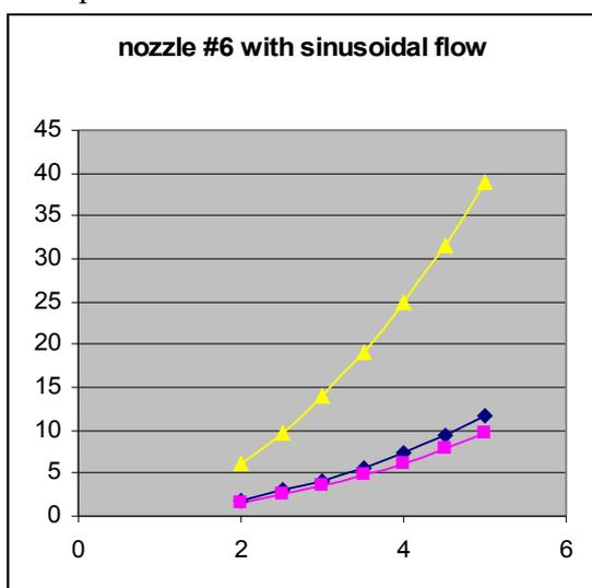
In purple the theoretical mean thrust versus frequency.
