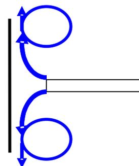
c) Then we placed some screens (chicanes) at various places inside the tank (not on the direct jet flow) and we saw a decrease of the thrust indication. The *right* thrust was got with a screen arranged as shown on the following scheme.
