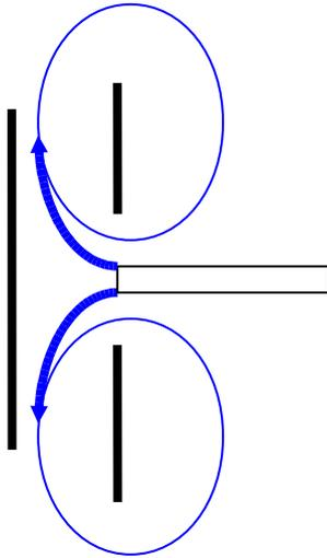
Such a screen doesn't prevent vortices, but they are large and the water which comes again towards the target has lost most of its velocity.
