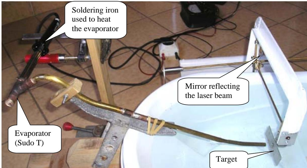
The soldering iron is powered through a dimmer. Voltage and current are measured to know the power.
