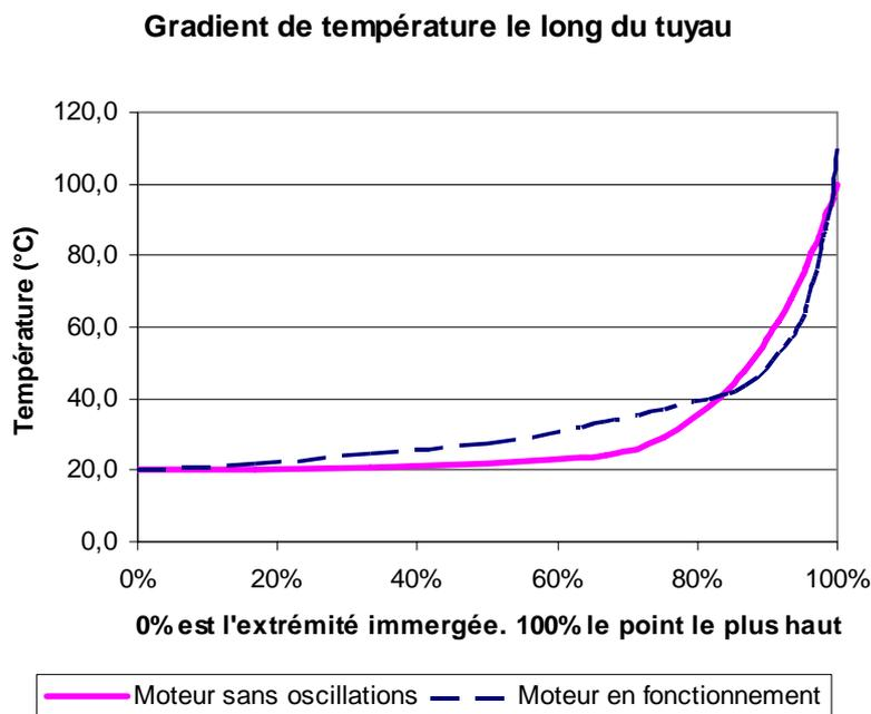
In blue dashes the measured gradient. Not measured on this engine, but measured on a smaller one and on a bigger one, both curves being similar. We just modify them slightly to refer to 20°C at the tank.
