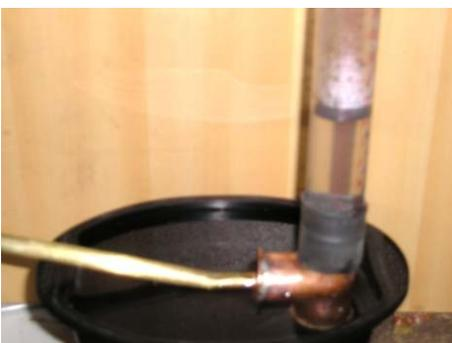
$14 \text{ g}$  for a piece of pipe of  $26 \text{ cm}^3$ . Therefore, without better knowledge, we can consider that when the engine runs well, the mass of water inside is approximately half the one that the falling part of the pipe can hold
