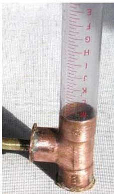
I reused a well known engine with electrical heating and I connected it to a Sudo T closed at the bottom and on its side by soldered lids. And on the top I connected a measuring test tube by means of a piece of bicycle inner tube.
