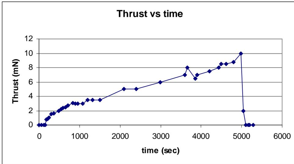
Compared with other engines, this one was running much more regularly (no burst of energy, no steam blast) up to (3600s, 7mN).
