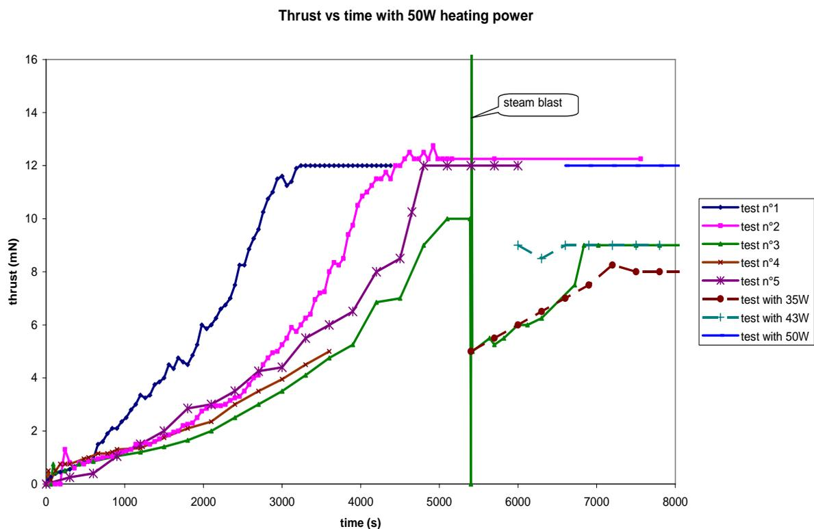
What worried us in a first approach is the fact the results (slope of the curves) differ from each other though the initial conditions were the same: same engine, same heating power, same temperature.
