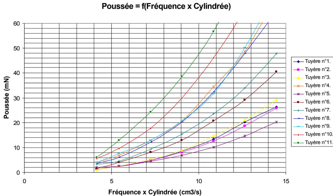
This graph shows thrust versus “frequency x stroke volume” for the 11 nozzles
