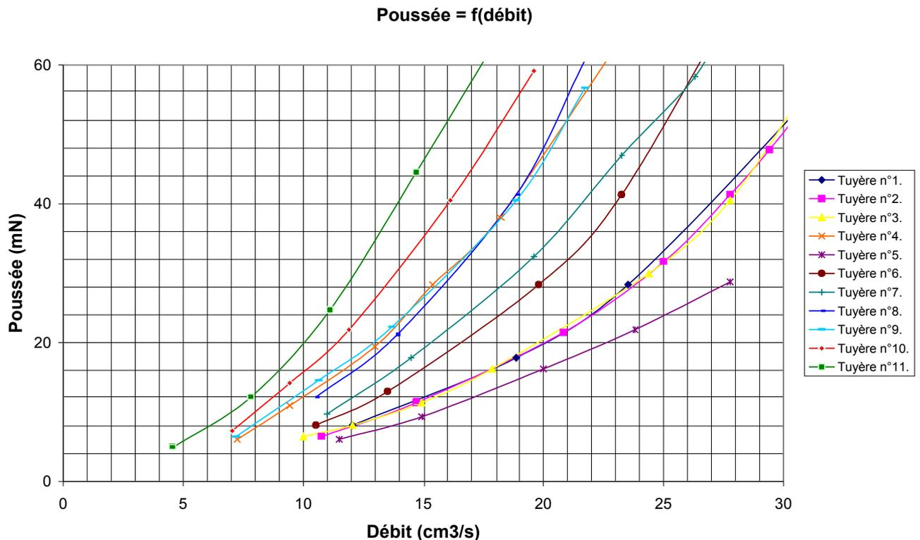
This graph shows thrust versus flow for the 11 nozzles.
