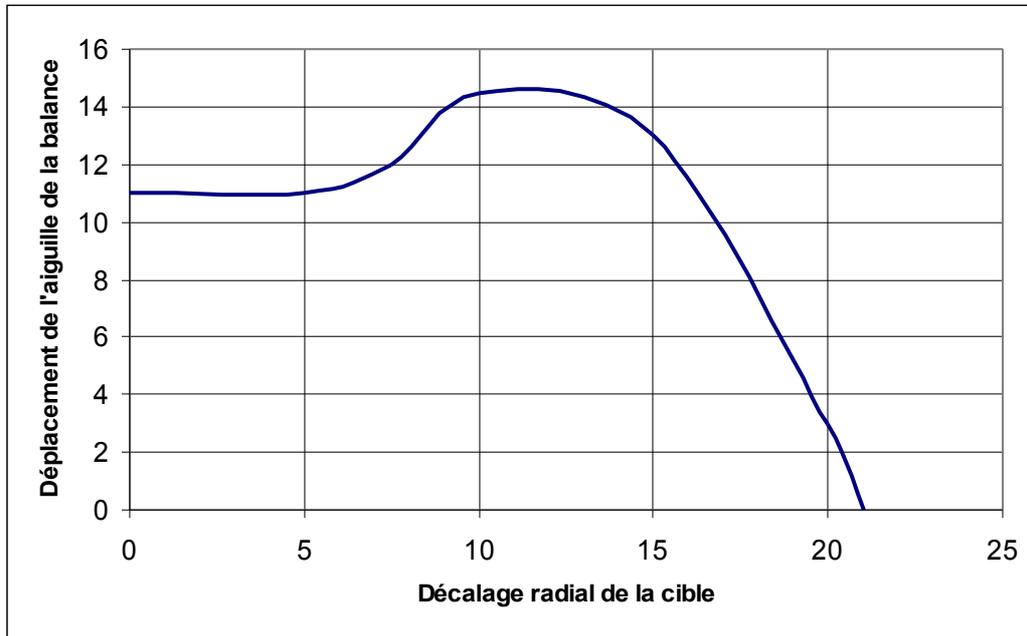
Similar curves were recorded at several distances between nozzle and target. This one was recorded with a 20mm distance.
