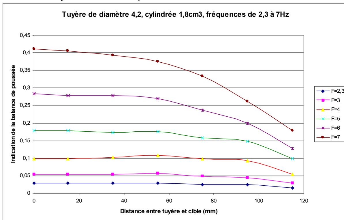
This graph shows the needle deviation versus distance for frequencies 2.3 to 7Hz. Stroke volume: 1.8 cm<sup>3</sup>. Nozzle diameter: 4.2 mm.
