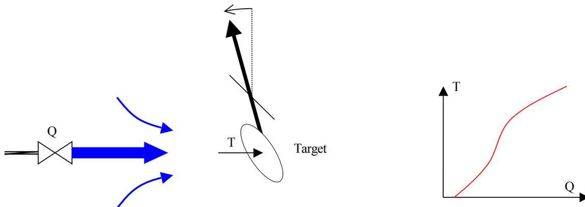
The thrust is not measured directly. In fact it is the deviation of the needle which is measured, but the torque needed to cause this deviation is known. See annex 2.
