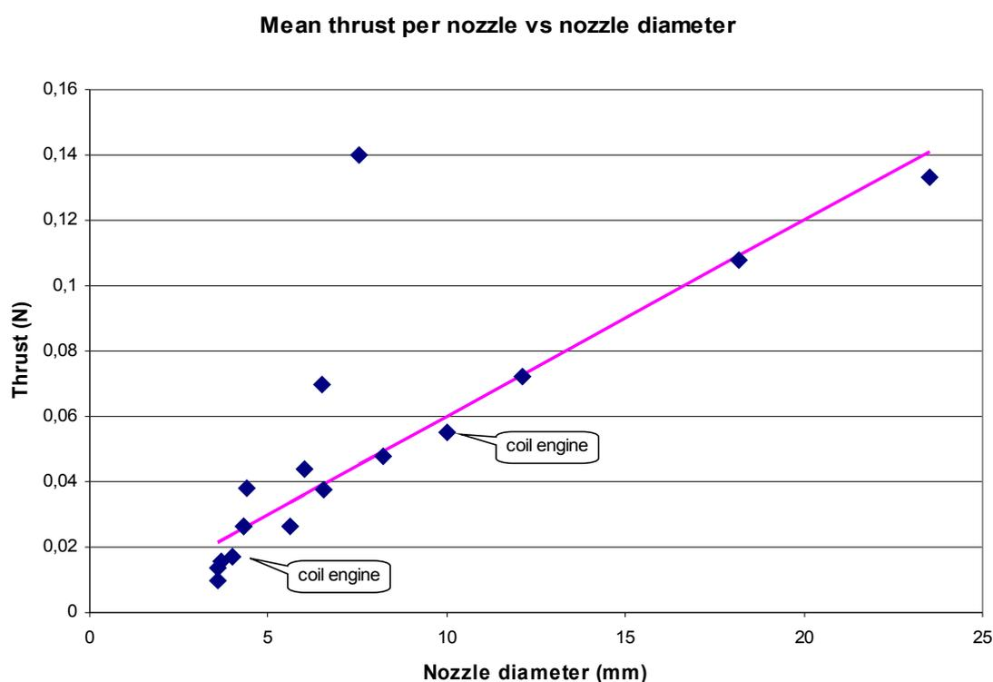
Note: what is called "mean thrust" is the average of a 15 minute record. Instantaneous thrusts up to 30 times higher than the average were recorded, but they are rare and they don't influence the average because they are generally followed by several seconds with no visible thrust.
