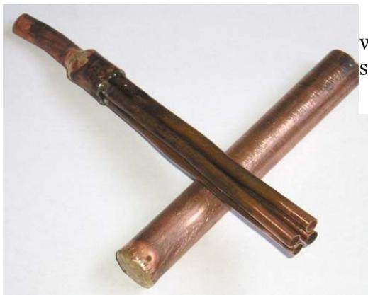
On a single pipe engine I tried an evaporator with pipes inside to increase the area of the hot source. Nothing bad or good to report.
