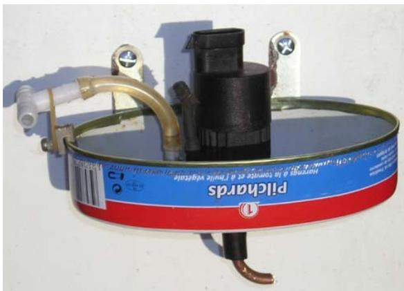
Sucking nozzle under the hull, cleared of the rest. Delivery above the water level (shared on both sides to avoid unwanted propulsive effects).
