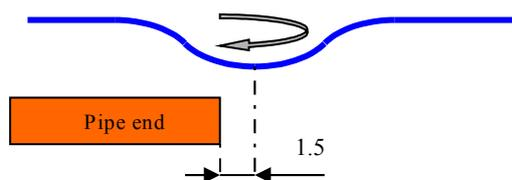
A small basin was created at the water free surface. Its centre was approximately 1.5mm ahead of the pipe. The water was rotating clockwise. (We are in the northern hemisphere).
