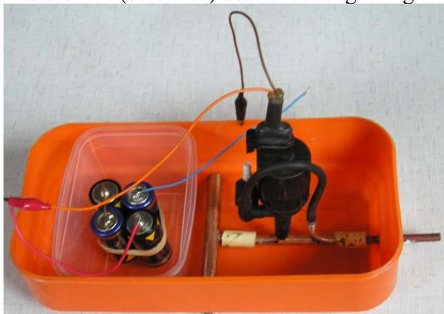
One can see on the left the batteries compartment, lower in the middle of the hull, the cross-over, in black, the pump, and on the right the tube used either to suck or to deliver.
