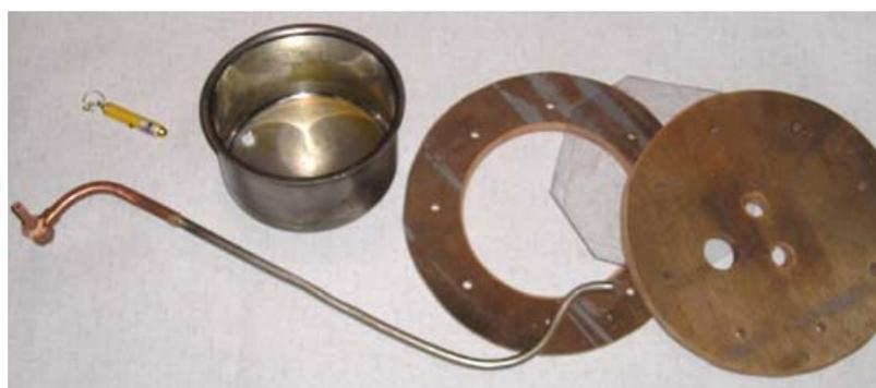
Note: the lower bends of the engine are due to the need of connecting it to the bowl at the bottom to allow the passage of the lower flange (made of plywood) after welding is completed.
