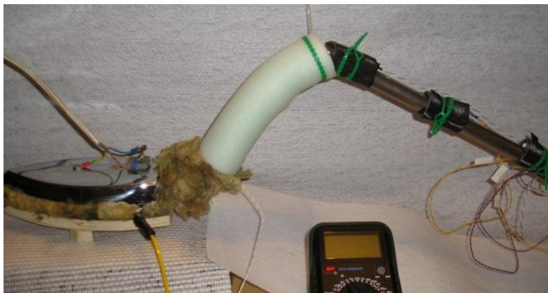
View of the engine isolated and provided with measuring instruments. The yellow wire is the one of a thermocouple measuring the copper pipe temperature. The grey one going out of the rock wool is the one of a thermocouple measuring the temperature of the boiler copper. The 3 black polystyrene sleeves cover PTC type temperature probes. This is a partial view of the engine. Totally there are 7
