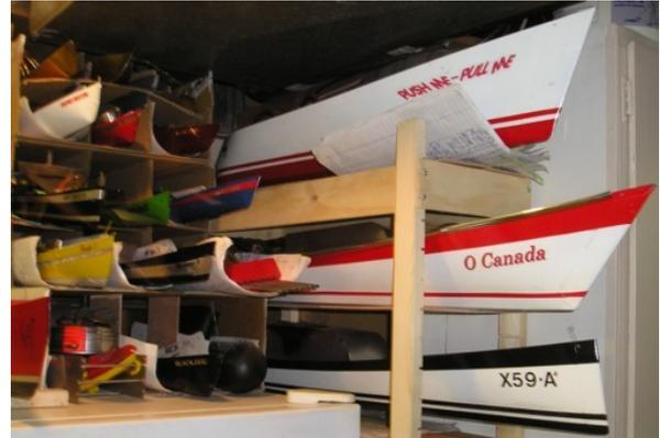
The boats are all different. They are built without drawing. Hulls are made of 20/100mm aluminum sheets; which makes them very light for their size.
