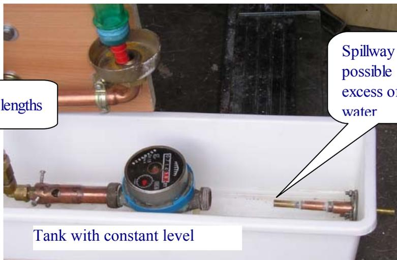
Spillway for possible excess of water
