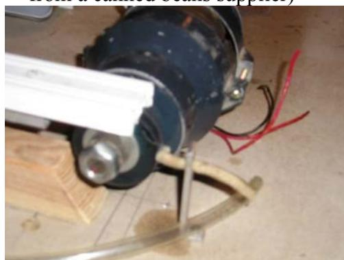
Cam (made of Lucite) and its lubrication (wick from an oil lamp soaked with oil)
