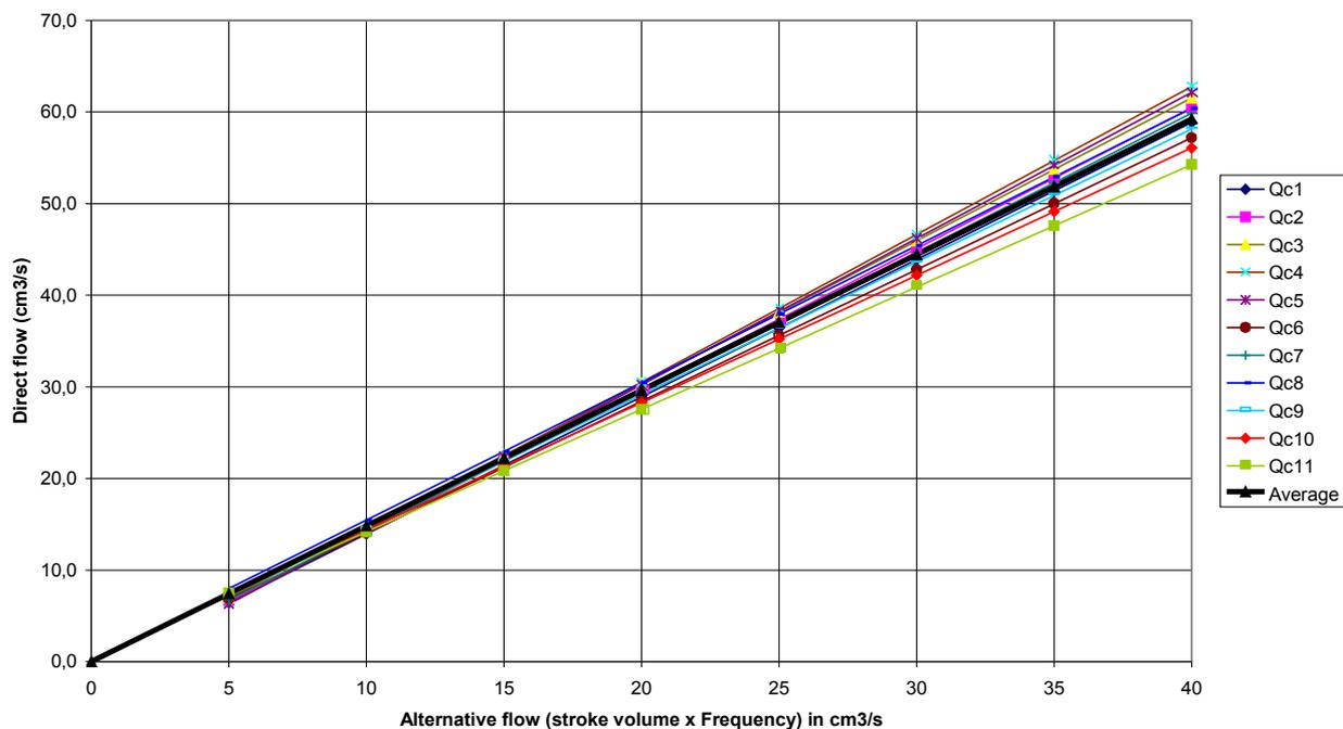
It was obvious a priori, but we can see on this graph, that (taking into account the inaccuracy) the curves are crossing the zero. As nothing was measured below 0.8Hz, we added the dot of abscissa zero and ordinate zero, and the average was calculated.
