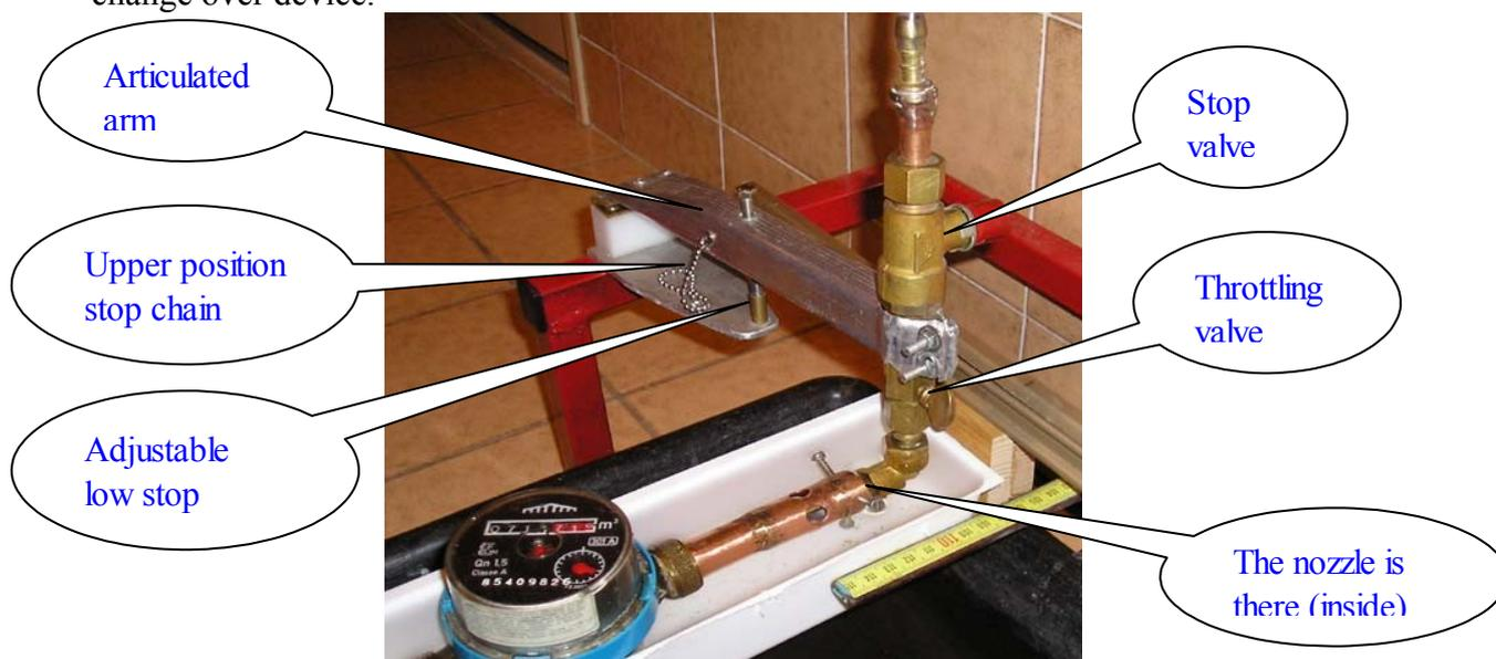
The (white) tank is horizontal and full, overflowing all along both sides. (No recirculation)
