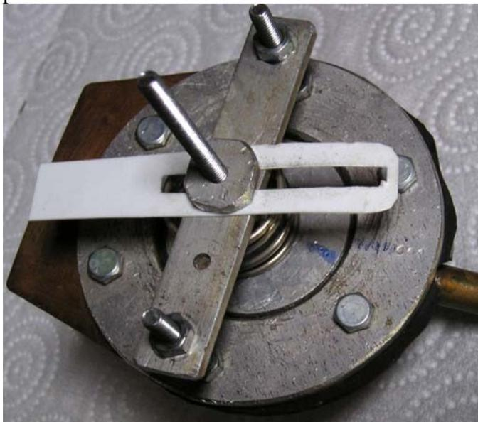
Note: At low pressures the accuracy is not very good because the diaphragm which is made of rubber has also a spring effect.
