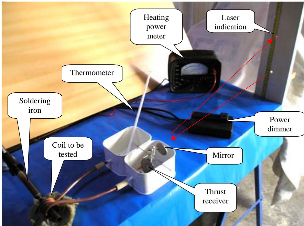
The laser emitter is located behind the vertical white board. The beam goes through a hole in the board. A rock wool mattress is visible below the coil. During the test another mattress was set above to limit heat losses.
