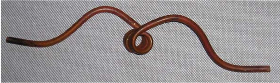
Later with the engine visible on the picture we measured a mean thrust of 12 mN (on each pipe) with peaks up to 18 for half a second. And this time, we could reproduce the result. A short record of this mean thrust is given above with the green curve. For more details look at the document “Test of a coil engine”.
