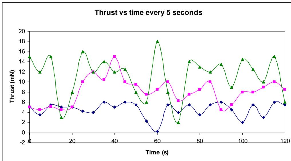
The best mean thrust measured with horizontal pipes was 9mN with peaks up to 13.5mN. The arrangement with horizontal pipes was very likely the cause of some of our difficulties to get a good steam liquid interface on both sides.
